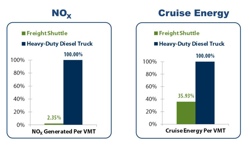
Note:  $NO_x$  emission factor of 11.89 g/VMT was used to estimate HDD truck emissions. An efficiency rating of 5.9 mpg was used to estimate HDD truck cruise energy.
